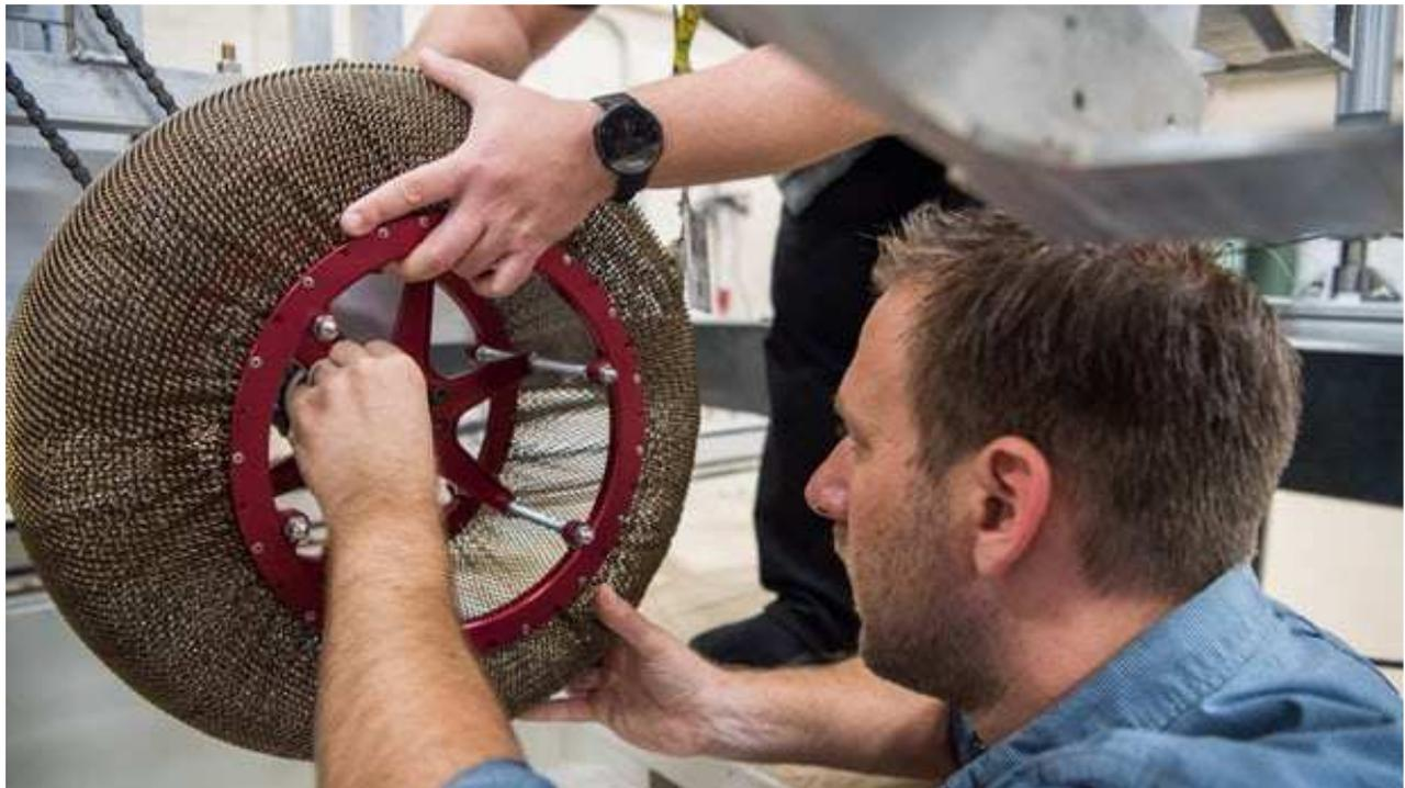
Constructing a test mesh tire(Credit: NASA)
