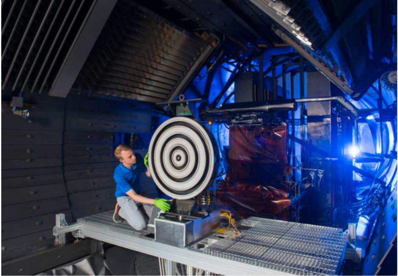
Scott Hall makes some final adjustments to the X3 ion thruster at the University of Michigan before a test. Credit: NASA
