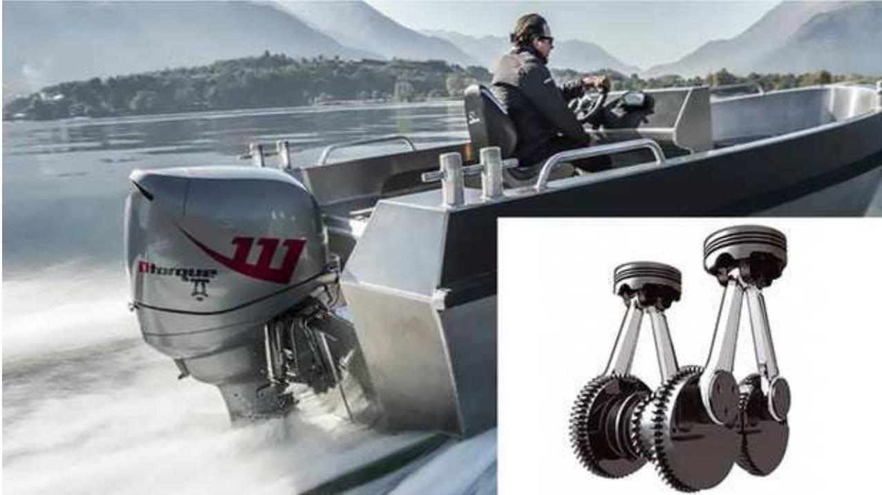
Compared to petrol outboards, the Yanmar is lighter, smoother, more compact, has double the engine life, and offers much better fuel consumption and running costs. It produces less toxic emissions, has more torque much lower in the rev range and that's before you consider the safety and ready availability of diesel fuel.(Credit: Yanmar/Neander-Motor)
