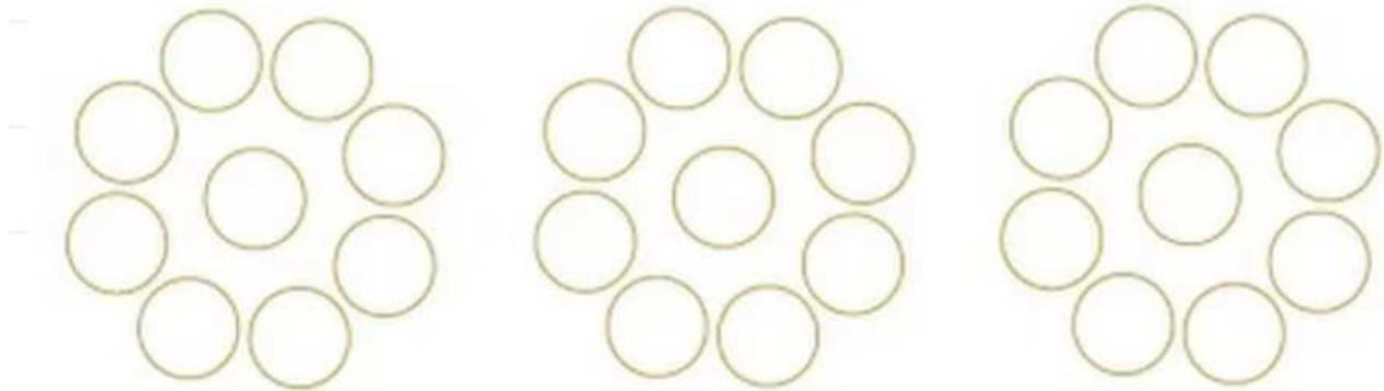
The 27 Merlin engines that power the Falcon Heavy's three cores are arranged in an "Octaweb" configuration. Credit: SpaceX
