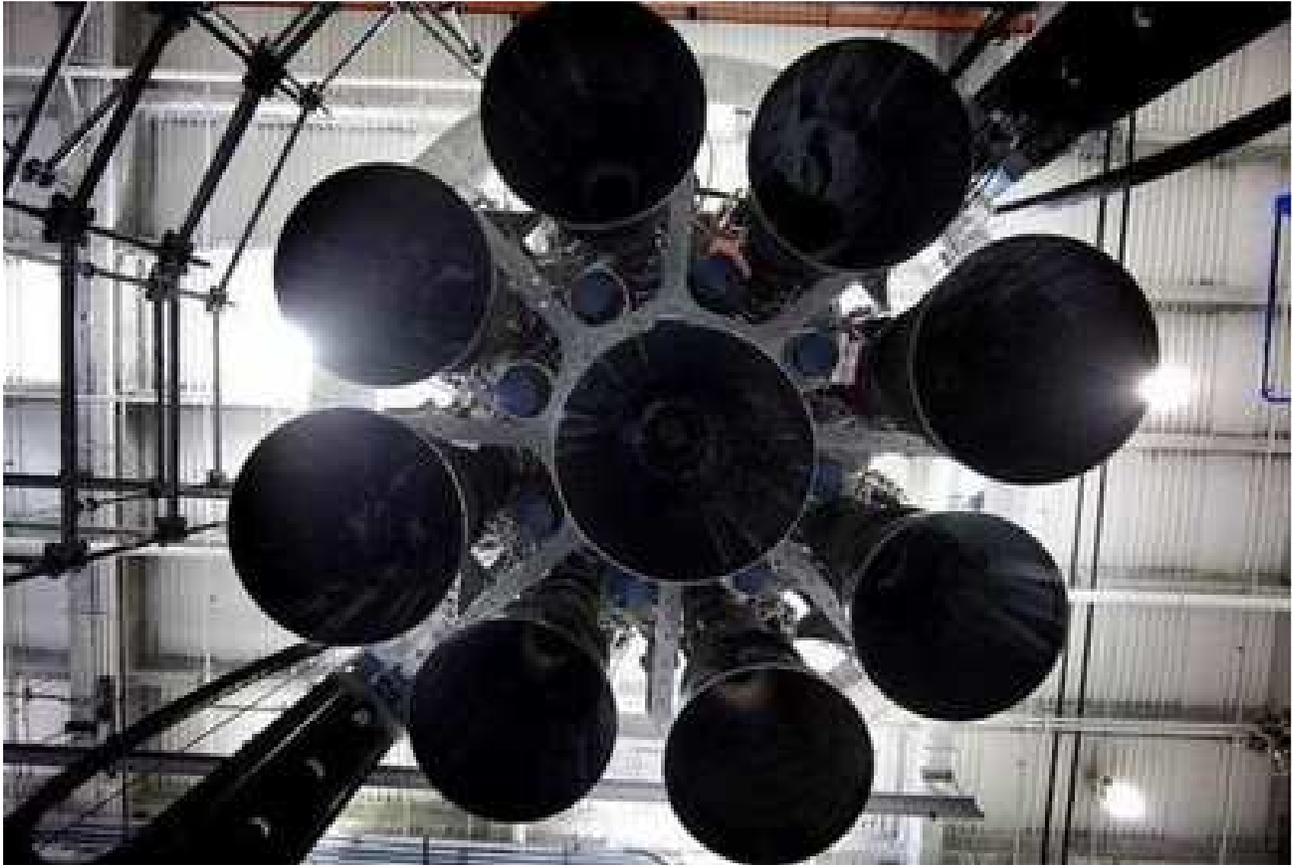
**Booster basics: The Falcon Heavy's Octaweb clustering of Merlin engines. Credit: SpaceX**
