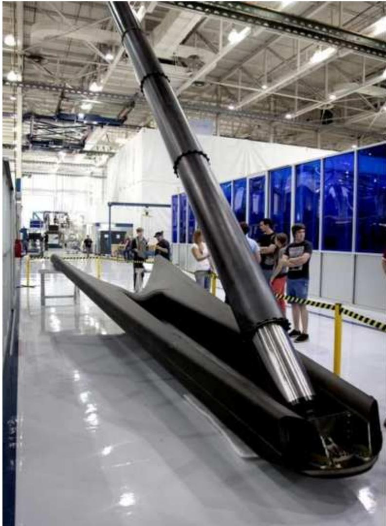
The Falcon Heavy was designed to be reusable. Both the center core and the side boosters carry landing legs, which will land each core on Earth after takeoff. Credit: SpaceX
