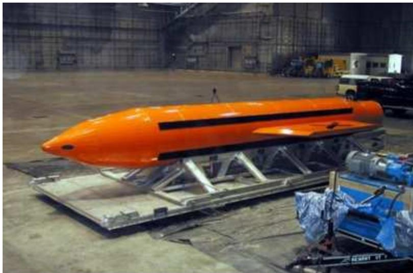
A Massive Ordnance Air Blast—or more commonly known as the "Mother of All Bombs" (MOAB)—weapon is prepared for testing at the Eglin Air Force Armament Center on March 11, 2003. The MOAB is a precision-guided munition weighing 21,500 pounds and will be dropped from a C-130 Hercules aircraft for the test. It will be the largest nonnuclear conventional weapon in existence. The MOAB is an Air Force Research Laboratory
