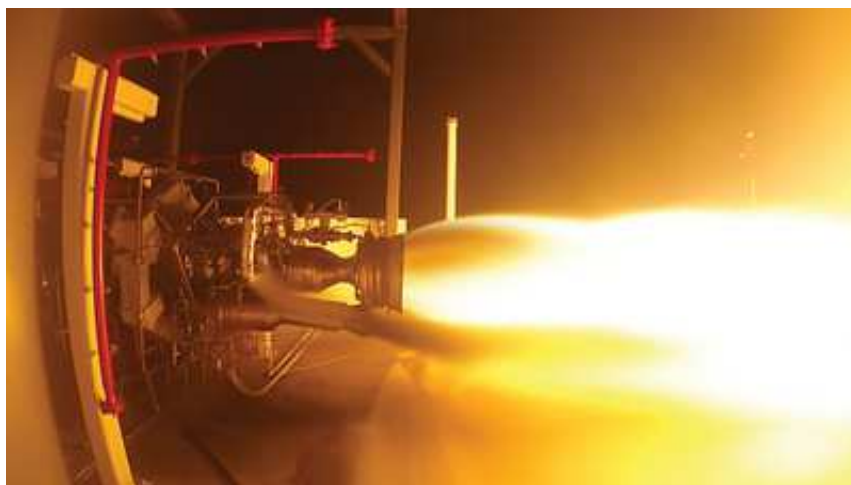
Firing of LauncherOne’s Newton Three liquid-oxygen/kerosene first-stage engine on Virgin’s test stand in Mojave, California. Credit: Virgin Orbit
