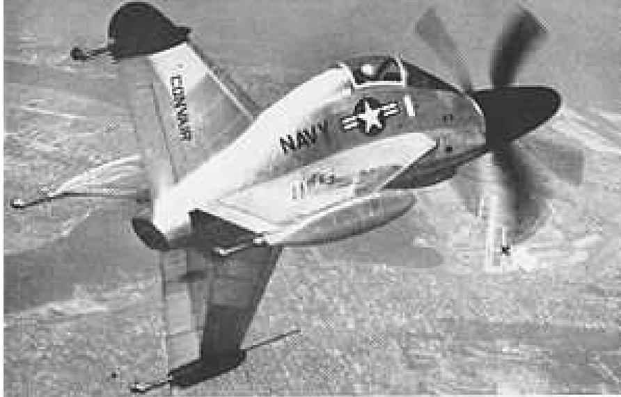
THE Convair XFY Pogo WAS A VTOL EXPERIMENTAL TURBOPROP AIRCRAFT FROM THE 50'S THAT WAS ABANDONED BECAUSE THE PILOT COULD NOT SEE BEHIND HIMSELF TO LAND THE AIRCRAFT. WITH COMPUTER CONTROLS AND VIDEO SYSTEMS, THIS WOULD BE A PIECE OF CAKE TO FIX AND PLAY WITH. TAKE A LOOK AT IT ON WIKIPEDIA.
