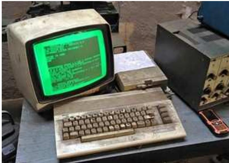
This Commodore 64 contains a few homemade aspects, however. The computer uses a sinusoidal waveform generator and piezo vibration sensor in order to measure changes in pressure, acceleration, temperature, strain or force by converting them to an electrical charge. The C64C interprets these signals to help balance the driveshafts in vehicles.
