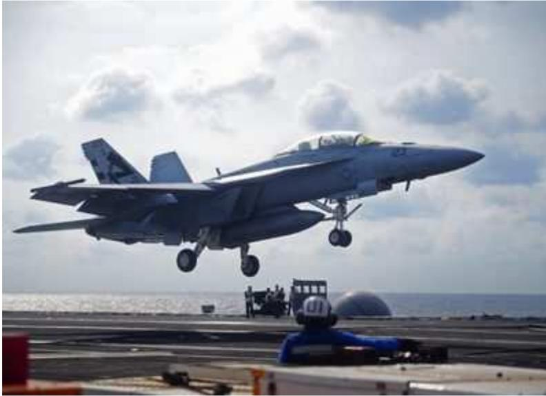
An F/A-18F Super Hornet from Air Test and Evaluation Squadron (VX) 23 performs a touch-and-go on the flight deck of the aircraft carrier USS George Washington. VX-23 is conducting tests of the Maritime Augmented Guidance with Integrated Controls for Carrier Approach and Recovery Precision Enabling Technologies (MAGIC CARPET). MASS COMMUNICATION SPECIALIST SEAMAN CLEMENTE A. LYNCH/U.S. NAVY
