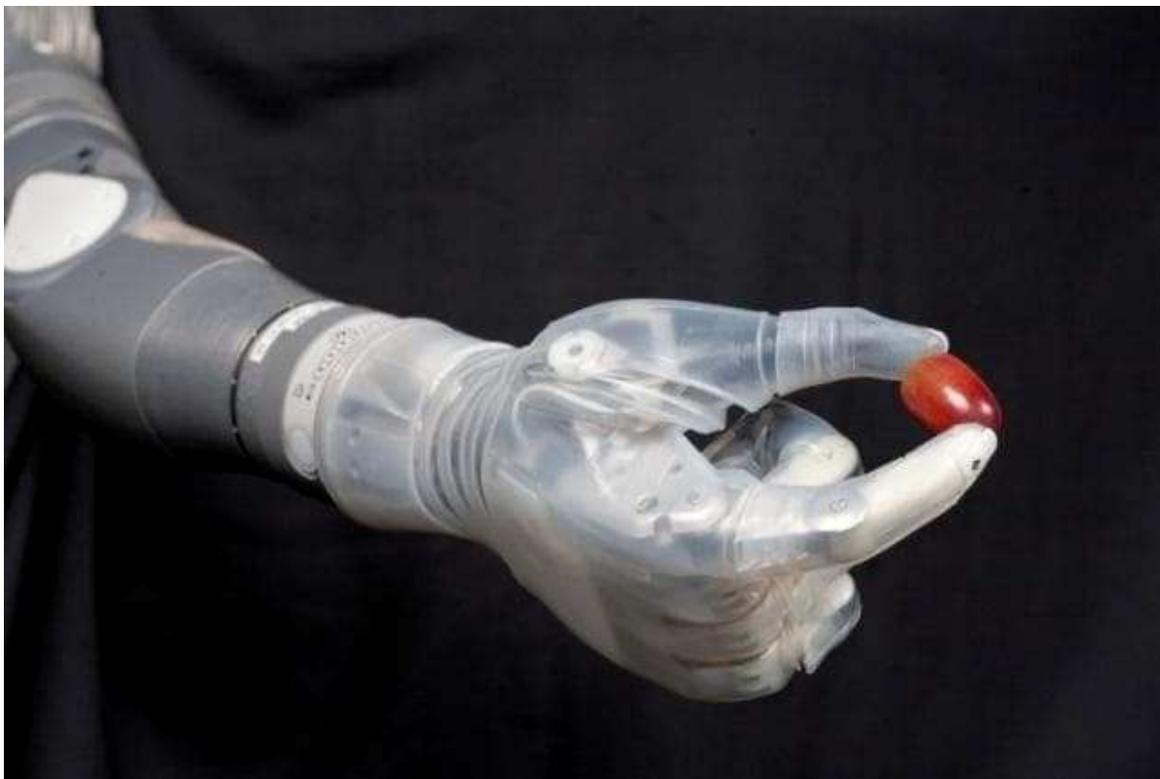
The system has a sensor that also returns "grip-force" information back to the patient, giving feedback about how firmly something is being grasped. Another new innovation is the use of foot-mounted inertial measurement sensors connected wirelessly to the arm that offer an alternative means of control.
