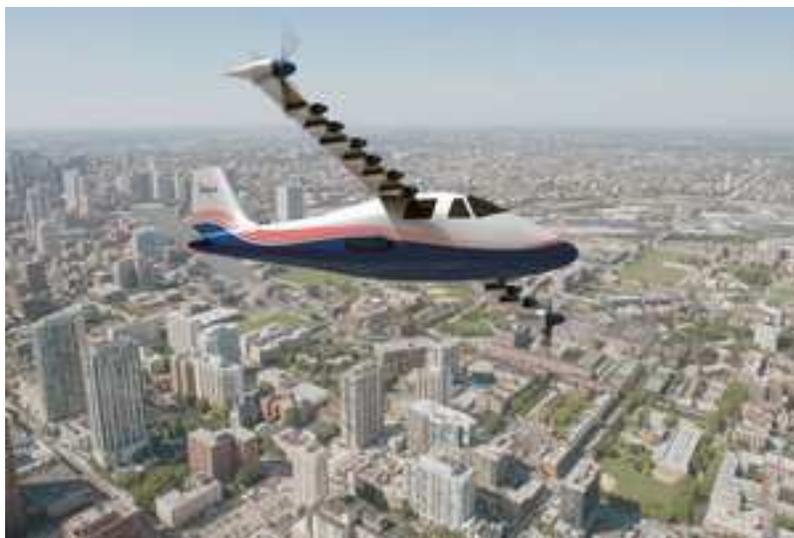
An artist’s concept of NASA’s X-57 Maxwell aircraft showing the plane’s specially designed wings and 14 electric motors. Credit NASA Langley/Advanced Concepts Lab, AMA, Inc.
