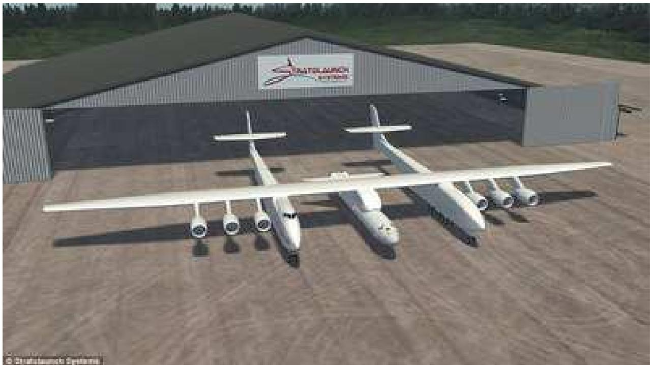
+11 Each of the twin fuselages of the Stratolaunch Carrier aircraft is 238 feet (72 metres) long and, when complete, will be supported by 12 main landing gear wheels and two nose gear wheels
