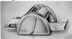
The Low Cost DITTO D-10 makes copies of anything you can type, write, trace or draw, in one to five colors at once, at a speed of up to 120 bright clear copies per minute. Takes any standard size or weight paper or card stock. Makes 10 copies for less than a penny!
